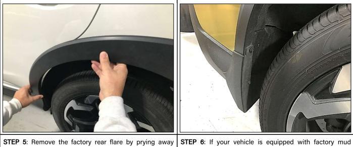
**STEP 5**: Remove the factory rear flare by prying away from the vehicle (this will disengage the plastic retainers holding the flare on the vehicle). Discard.
