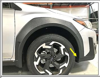
**STEP 15**: Install 8mm push in clip into the lowest forward hole drilled in step 8.
