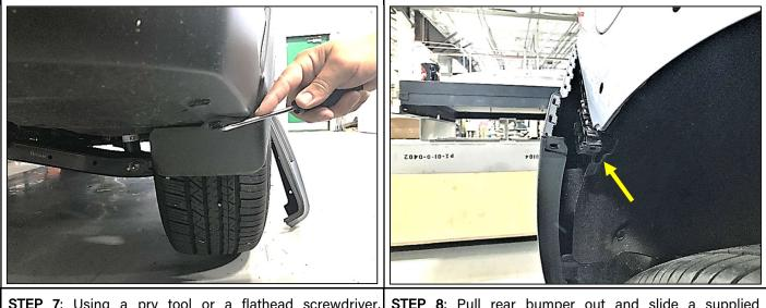
STEP 7: Using a pry tool or a flathead screwdriver,<br/>remove plastic retainer from underside of factory mud flap.STEP 8: Pull rear bumper out and slide a supplied<br/>Narrow "U" Clip onto the plastic bracket as shown. Push<br/>bumper back into alignment.
