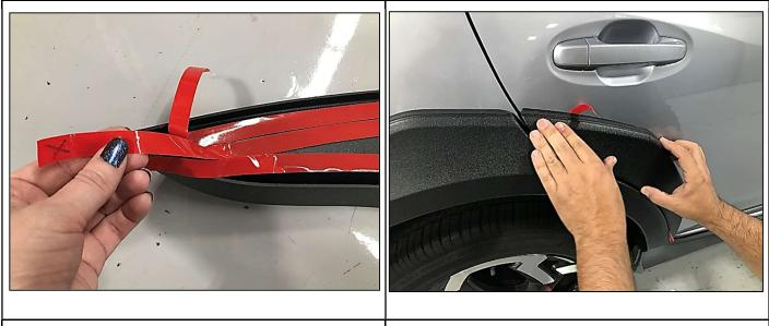
**STEP 17**: Mark the liner for the center tape piece on the door piece, then fold out all tape liners so that they will be accessible. During installation, this center liner **must** be pulled *before* the outer liners or you will not be able to remove all the tape liners.
