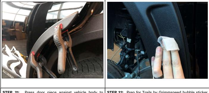
**STEP 21**: Press door piece against vehicle body to completely adhere tape once liner is peeled. Use 2-3 spring clamps to hold piece in place during bonding (for a total of 5 minutes). Tape bonds fully within 24 hours at 60 degrees F.
