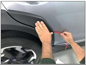
**STEP 20**: Making sure the door piece is properly aligned, carefully peel tape liner from tape incrementally, starting with the center liner marked in step 17. NOTE: If the part slips in the early stages of taping, it is possible to move it if needed. Once part is adhered enough to stay aligned, press as you go.
