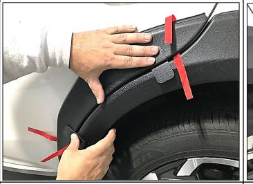
**STEP 19**: Use 2 supplied door spacing tools to align door piece with rear flare, maintaining uniform gap along seam.
