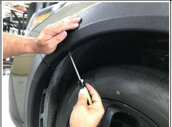
STEP 13: Install supplied screws through seven (7) holes in flare and into clips installed in previous steps. Install factory bolts into factory mud flap clips if present.
