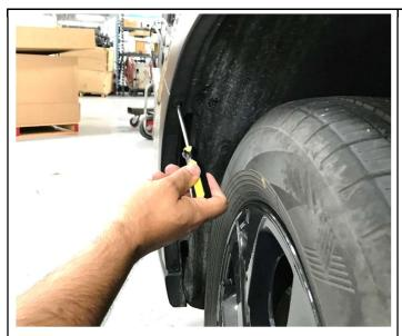
**STEP 7**: Bumper cladding removal: Using Phillips screwdriver, push two (2) plastic retainers at front of wheel well inward toward bumper to disengage (retainers will click when disengaged).
