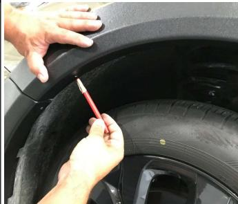
**STEP 9**: Install two (2) supplied plastic-panel clips over factory holes in bumper.
