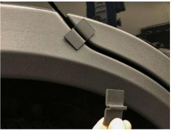
STEP 16: Use 2 supplied door spacing tools to align door piece with rear flare, maintaining uniform gap along seam. (NOTE: it may be helpful to apply a small amount of tape to hold spacers in place during install.)
