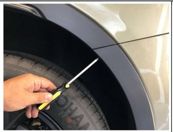
**STEP 7**: Using Phillips screwdriver, push one (1) plastic retainer located at upper rear of wheel well toward vehicle body to disengage (retainer will click when disengaged). Do not remove plastic retainer at lower rear of wheel well or rear cladding.
