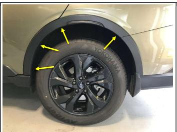
**STEP 11**: Install four (4) supplied plastic-panel clips over holes drilled in step 10.
