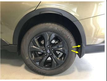
**STEP 6**: If factory mud flap is not present, peel back wheel well liner and install two (2) supplied plastic-panel clips over two (2) outer factory hole locations in rear of wheel well. The flat side of the clip will be at the wheel well side.
