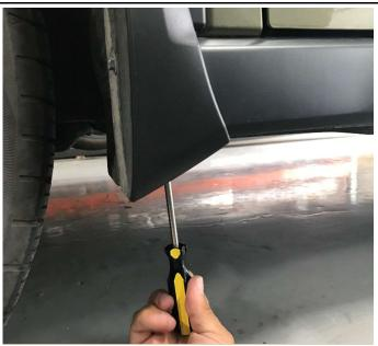
STEP 4: Remove one (1) factory bolt from underside of mud flap using 7/16" / 12mm socket. Discard.
