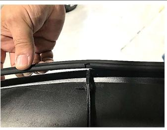
**STEP 2**: Install supplied edge trim on assembled front flare, cutting a "U" notch when you reach the main/bumper piece assembly connection point.
