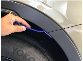
**STEP 8**: Using trim removal tool, remove plastic retainer and discard. Install one (1) supplied plastic-panel clip over factory hole vacated by plastic retainer.
