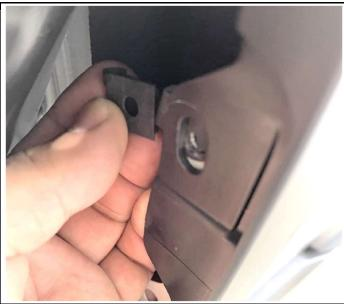
STEP 6: If factory mud flap is not present, peel back wheel well liner and install two (2) supplied sheet metal clips over two (2) outer factory hole locations in rear of wheel well. The flat side of the clip will be at the wheel well side.
