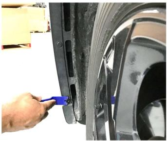
**STEP 8**: Using a trim removal tool, remove three (3) plastic retainers. Pry plastic bumper cladding piece from vehicle, disengaging three (3) plastic tabs located inside cladding piece. Discard cladding and plastic retainers.
