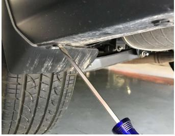
**STEP 4**: Using trim removal tool or flathead screwdriver, remove one (1) plastic retainer underneath mud flap and another inside wheel well. Discard retainer.
