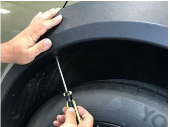
**STEP 12**: Install supplied screws through seven (7) holes in flare and into clips installed in previous steps, and factory bolts into factory mud flap clips if present.
