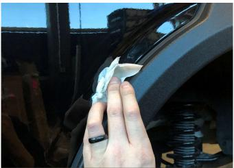
**STEP 13**: Ensuring continued fit of flare against fender, tighten all screws/bolts.
