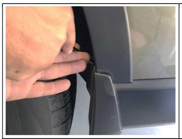
**STEP 5**: Remove mud flap from vehicle and discard. There will be two (2) factory clips installed on fender underneath mud flap – keep these in place.
