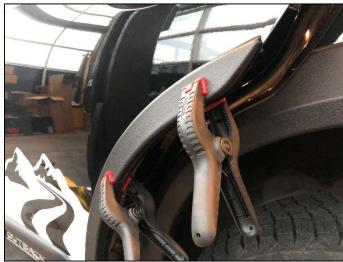
STEP 17: Making sure the door piece is properly aligned, carefully peel tape liner from tape incrementally. NOTE: If the part slips in the early stages of taping, it is possible to move it if needed. Once part is adhered enough to stay aligned, press as you go.
