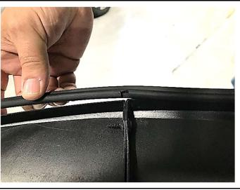
**STEP 2**: Install supplied edge trim on assembled rear flare, cutting a "U" notch when you reach the main/bumper piece assembly connection point.
