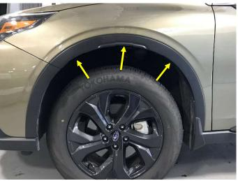
**STEP 12**: Install three (3) supplied plastic-panel clips over holes drilled in step 11.
