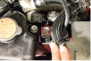
2. Remove the 10mm and 12mm bolts so that the 0EM cover can be flipped upside down to reveal the nut and bolt underneath.
