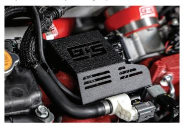
**Note:** We recommend using The GrimmSpeed EBCS with this cover. If you are still using the OEM Boost Control unit, it can mount underneath the cover using the factory hardware as shown below.
