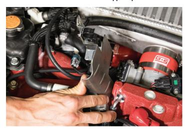
3. Remove the 10mm nut on the underside of the cover and the mounting bolt that holds the BCS to the 0EM cover (Our car is equipped with the GrimmSpeed 3-Port Boost Control Solenoid).
