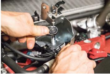
4. Once all bolts are out you should be able to remove the OEM cover from the engine bay.
