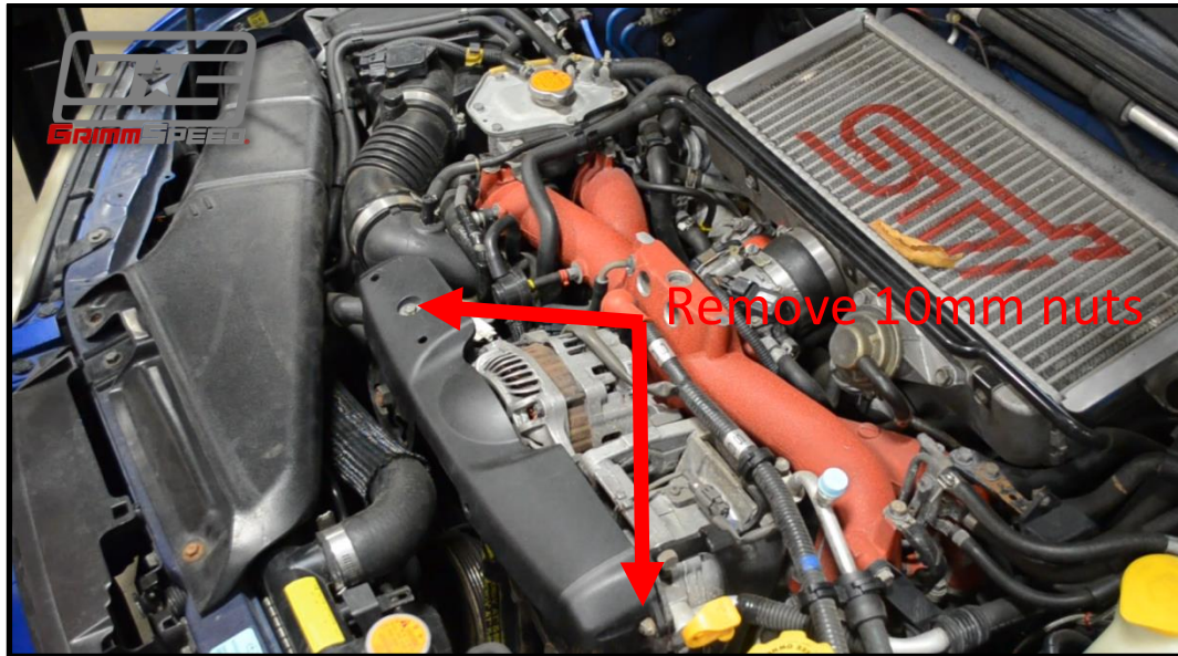
Figure 2: Remove 10mm nuts on each side
