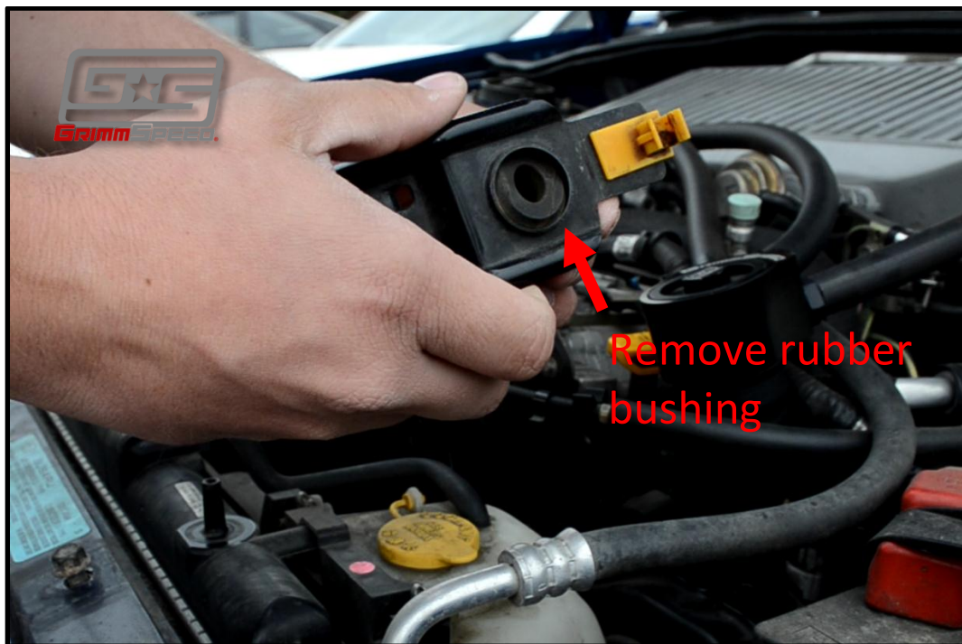
Figure 5: Removing rubber bushings
