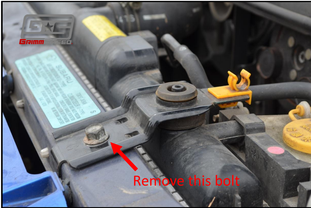
Figure 3: Remove OEM radiator stay brackets
