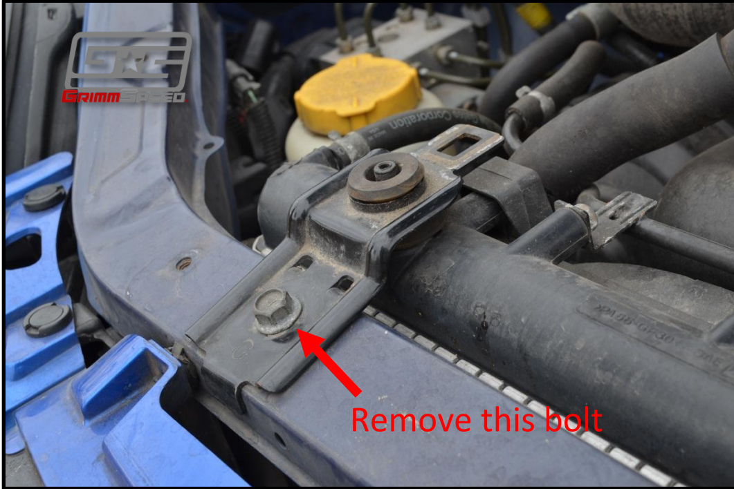
Figure 4: Remove OEM radiator stay brackets
