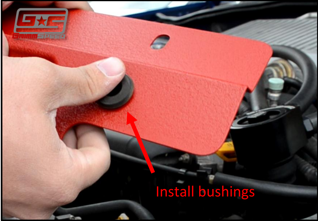
Figure 8: Install rubber bushings
