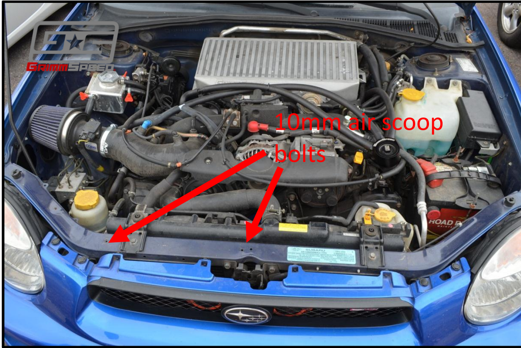
Figure 2: Air scoop bolt locations
