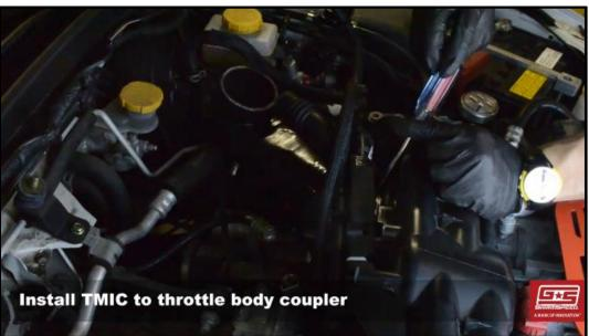
20. Repeat the process on the passenger side, installing the coupler such that when looking straight down at it, it appears thinner. Leave this clamp loose for the moment.
