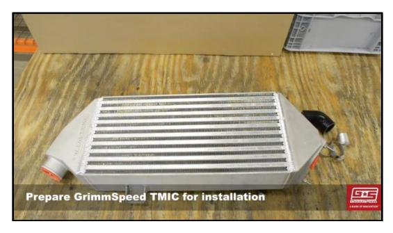
22. Finally, position the intercooler in the engine bay, lining up the tab in the rear with the rear bracket and then the front. It should drop into position nicely. Manipulate the intercooler and the silicone couplers so that the couplers are securely over each side of the intercooler. Tighten worm gear clamps.
