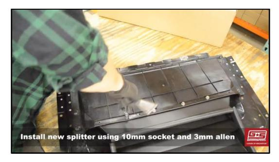
6. Reinstall the updated splitter assembly onto the hood of the car using the six (6) Phillips head screws and five (5) push clips. Note that the rear of the splitter has two small tabs that slide into the hood and hold it in place. Be sure that these are in position before fastening the splitter.
