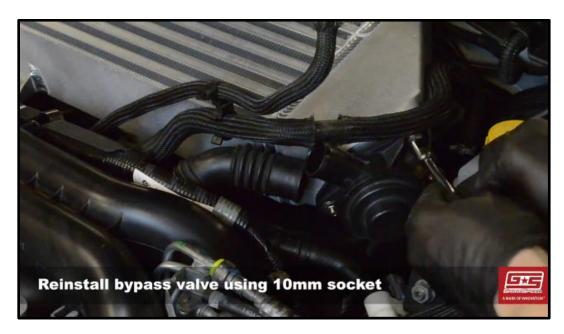
24. Next we'll install the BPV hose extension. If you have an aftermarket BPV hose, you should use the supplied aluminum tube as a coupler. If you have the stock hose in place, slide the aluminum tube into the stock hose as shown. A small plastic lip will stock it from dropping in. Next, install the GrimmSpeed silicone extension onto both the hose and the bypass valve using the supplied worm gear clamps.
