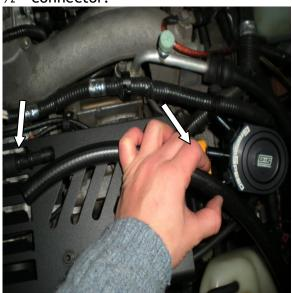
6. Using supplied hose(cut to fit), connect right bottom port on AOS with TMIC hard pipe:
