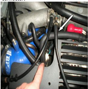
5. Using ~10" of supplied hose, connect upper port of AOS (middle one) to the other side of the  $\frac{1}{2}$ " connector.
