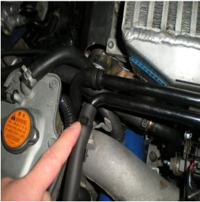
4. Position the disconnected hose to face towards the oil cap. Connect supplied plastic  $\frac{1}{2}$ " connector.
