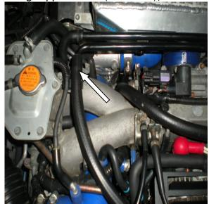
7. Pull OEM Hose that connects crankcase "T" to turbo inlet hose off of the turbo inlet. Push in ½" to ½" connector into oem hose. Connect supplied ½" hose to other end of ½" connector and bring to left bottom port on the AOS. Cut ½" hose to size and push on AOS hose fitting.
