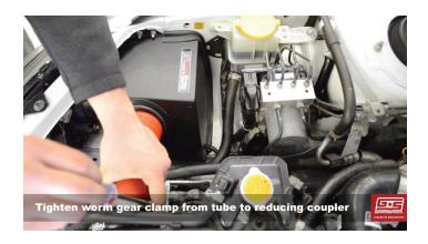
22. You may need to adjust the rotation of the intake tube slightly, to ensure that it's not rubbing on other hoses.
