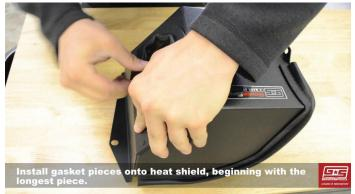
13. Next, assemble the heat shield with the intake tube.
