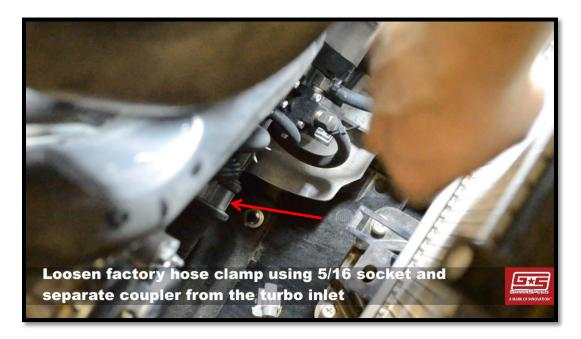
11. With the bottom portion of the factory intake separated from the plastic turbo inlet, you can now move back to the remaining portion of the airbox and maneuver it out of the engine bay. You'll need to do some twisting and take advantage of the accordion flexible sections.
