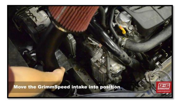
19. Reach down and slip the included worm gear clamp over the opposite end of the hump hose coupler loosely and slip the GrimmSpeed intake into place on the plastic turbo inlet. Do not tighten this coupler yet – we want some wiggle room for the next step.
