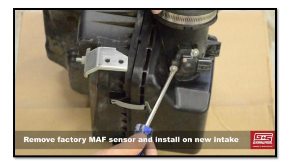
14. Reinstall your MAF sensor into the new GrimmSpeed tube using the included machine screws and your 3mm allen wrench. The MAF can only be installed in one direction, so there's no need to worry about accidentally installing it backwards.
