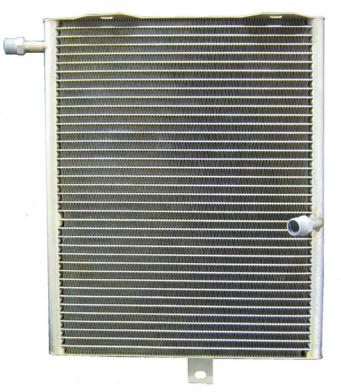
The new Porsche 930 Kuehl High Performance Condenser for the 930 turbo deck lid is a direct drop in, bolt on, replacement for the stock factory condenser. This new condenser utilizes the latest generation "plate and fin" tubing technology. The benefits of the Kuehl design lay in its twin (double) manifolds with thin multi-channel extrusions and high fin density.
