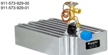
Griffiths' high performance Kuehl Serpentine Evaporator is a drop in replacement for the old-style tube and fin evaporator. The Kuehl Evaporator has only 2 brazed joints which reduces chances for leaks. The cooling fins are permanently brazed to the serpentine extruded tube which insures greater heat transfer.
