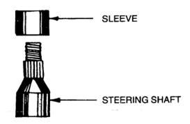
AFTER THE EXISTING STEERING WHEEL AND ASSOCIATED HARDWARE HAVE BEEN REMOVED AS INDICATED IN YOUR INSTRUCTION SHEET PLACE SLEEVE OVER STEERING SHAFT AS SHOWN ABOVE.
