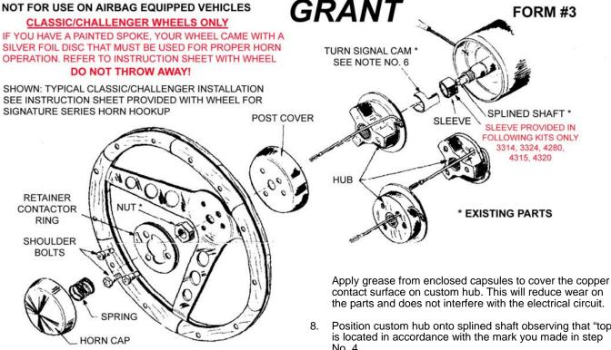
ATTN: TOYOTA (HUB NO. 10179) AND HONDA/ACURA VEHICLES (HUB NO. 10069). THESE HUBS ARE DESIGNED TO FIT ONTO THE SHAFT VERY TIGHTLY AND BE DRAWN DOWN BY TIGHTENING THE SHAFT NUT.
