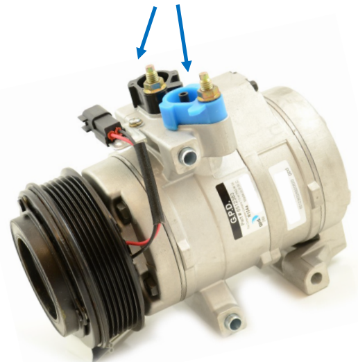
gpd #6512363 Hose fitting bolts on the right
