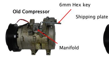
2. Remove the 2x6mm bolts using caution as compressor may be under pressure. Remove manifold from old compressor taking care not to get any dirt inside manifold. If concerned, clean dirt away. 3. Place new compressor facing the same way as the one removed from the vehicle. Locate shipping plate on top of compressor. Undo 2x6mm hex
