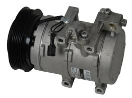
6. Place manifold from old compressor on to your new compressor and tighten. *Caution!* Make sure the manifold is in the right direction, it will fit on the compressor backwards and will have a dramatic effect on the performance of your new compressor. Ensure the manifold is put on the new compressor in the same place/location as when it was taken from the old one.
