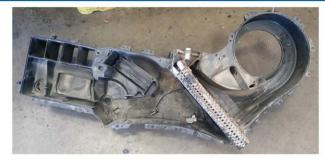
gpd has noticed an issue with 2009–2014 Ford F–150 pickups pertaining to their evaporator. Ford sells the unit as a total assembly but it has been designed to be split and put back together with screws. *The replacement evaporator is gpd #4712009.*
