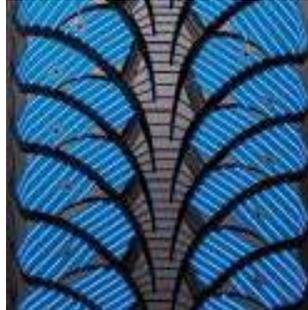
Three-dimensional TredLock Technology blades in the shoulder zone offer enhanced wet and winter traction, locking together for confident grip in turns.
