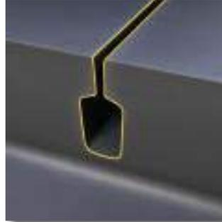
Evolving Traction Grooves help maintain confident traction in rain and snow as the tire wears.
