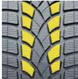
High-amplitude sipes enhance lateral stability for confident handling in wet and slushy conditions.
