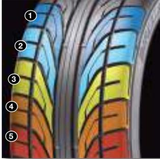
5-Pitch Technology counterbalances vehicle disturbance while minimizing road and pass-by noise. Five different block sizes create various frequencies to help break up sound waves, so drivers can enjoy a quiet ride.
