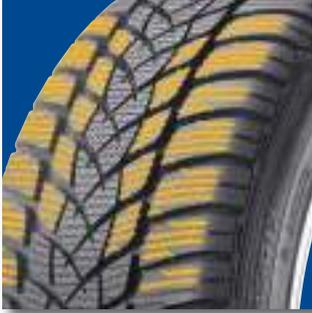
Adaptive SipeGrip Technology helps enhance gripping power under slippery conditions while maintaining dry and wet handling.
