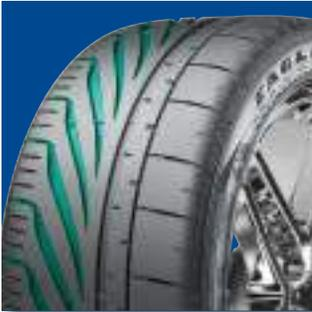
Sweeping Aquachannel Grooves on the inboard side of the tread help enhance wet cornering grip.
