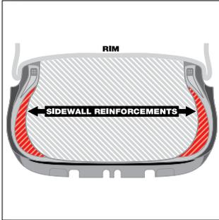
Dunlop Self-Supporting Technology incorporates special reinforcements into the tire sidewalls so that driving may continue for up to 50 miles at speeds up to 50 mph, even after a complete loss of air pressure. Refer to the run-flat owner's manual/limited warranty recommendations on operation at low or no air pressure. Tire pressure monitoring system required. Sold separately.
