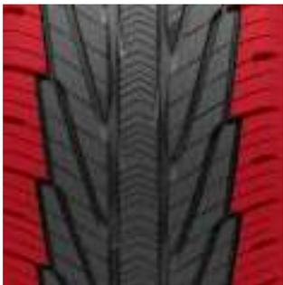
Dry Zone has large tread blocks along the outer edges to help provide confident handling on dry roads.
