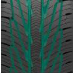
Water Zone has a sweeping tread pattern that helps evacuate water away from the tread for enhanced wet traction.
