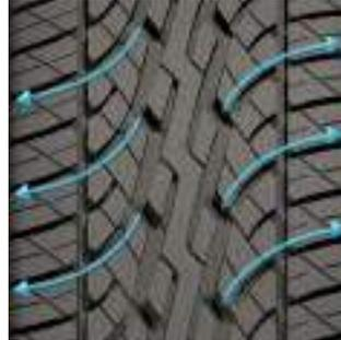
Angled Evaqua Grooves are situated to help efficiently evacuate water away from the footprint for responsive handling on wet roads.
