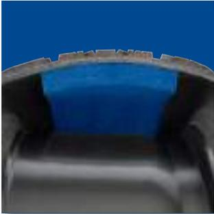
Polyurethane foam bonded to the tire's inner surface helps to reduce the level of interior vehicle noise, offering passengers a quieter, more comfortable ride.
