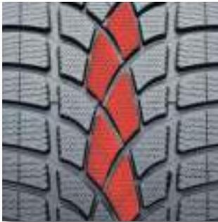
The center-block sipes help "pull," which results in superior traction and braking on ice and snow.
