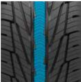
Ice Zone has numerous biting edges offering enhanced gripping traction on icy and slick roads.
