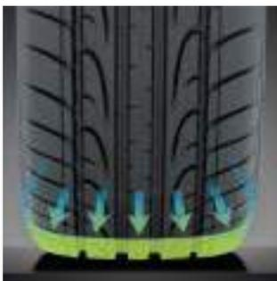
Innovative Multi-Radius Tread Technology distributes pressure evenly over the contact patch through all stages of cornering, for excellent dry traction and handling while enhancing wet performance.
