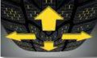
An increased number of sipes across the tire spectrum help provide extra traction during winter conditions. With self-interlocking and transversal sipes, the 4D Sipe System was specifically designed to enhance snow handling performance.
