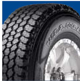
Durawall Technology helps resist cuts and punctures to sidewalls.
