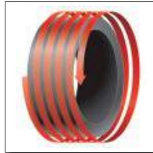
Jointless Band Technology helps maintain the tire's shape at highway speeds. With fabric positioned in all the right places to enhance handling and treadwear, this continuous spiral ply serves to help reduce vibration.
