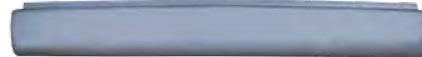
81-87 Chevy Pickup Front roll pan w/o license plate box Not EDP coated • EFXRP01
