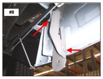
**STEP-9** <u>ATTACH THE DRIVER SIDE STEP</u> TO THE FRONT AND REAR BRACKETS USING (1) 1/2" X 2" HEX BOLT, (1) ½" FLAT WASHER AND (1) 1/2" LOCK WASHER FOR EACH BRACKET.
