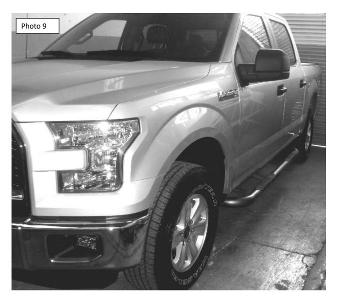
7. Align the side bar with the vehicle and tighten all brackets and side bar nuts and bolts. (Photo 9)
