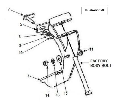
Step-5 Remove the passenger side rear body mount bolt, (Photo 5).
