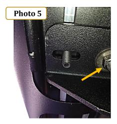
**Step-9** Align the side step with the vehicle and tighten all brackets and side steps nuts and bolts. Repeat the above steps to install the passenger side brackets and side step. Remember to check and retighten the nuts and bolts every six months.
