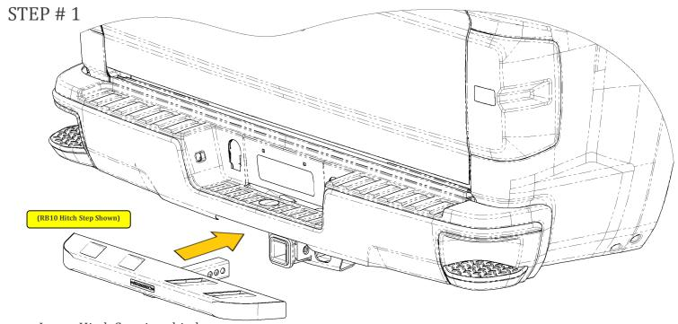
Insert Hitch Step into hitch.
