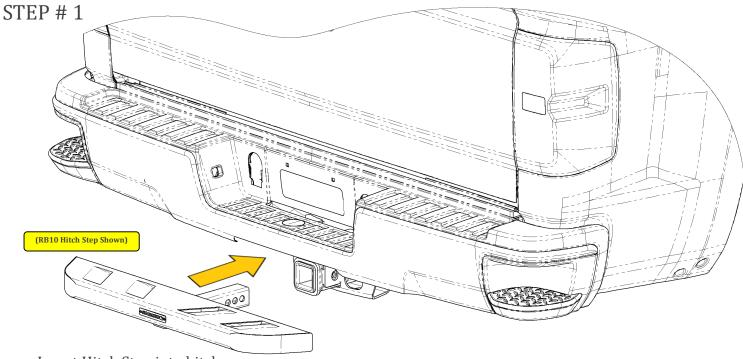
• Insert Hitch Step into hitch.
