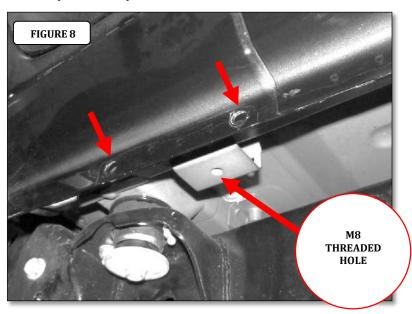
**Step-6** Attach one of the passenger side rear brackets to the pinch mold using (2) 1/4" x 1" hex head bolts, (4) 1/4" flat washers, (2) 1/4" lock washers and (2) 1/4" hex nuts, and to the underside of the body using (1) M8 x 25mm hex bolt, (1) 5/16" lock washer and (1) 5/16" flat washer, (FIGURE 9 & 10).
