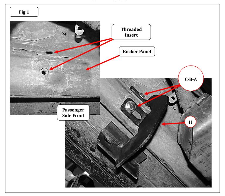
**Step-2** Locate the threaded inserts on the inner rocker panel at the center and rear of the cab and repeat step 1 to install the brackets using the supplied hardware. Note: The front mounting location is shown in Figure 2. The center and rear mounting locations are similar.
