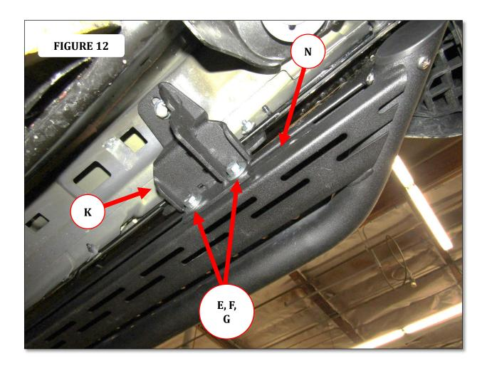
**Step-10** Align the Dominator D6 running board with the vehicle and tighten all bolts securing the running board to the front center and rear brackets. Repeat the above steps to install the passenger side brackets and running board. Remember to check and retighten the nuts and bolts every six months.
