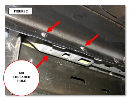
**Step-2** Attach the driver side Front bracket to the pinch mold using (2) 1/4" x 1" hex head bolts, (4) 1/4" flat washers, (2) 1/4" lock washers and (2) 1/4" hex nuts, and to the underside of the body using (1) M8 x 25mm hex bolt, (1) 5/16" lock washer and (1) 5/16" flat washer, (FIGURE 3 & 4). Leave the
