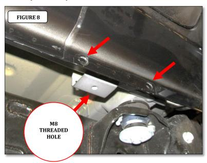
**Step-6** Attach the driver side Rear bracket to the pinch mold using (2) 1/4" x 1" hex head bolts, (4) 1/4" flat washers, (2) 1/4" lock washers and (2) 1/4" hex nuts, and to the underside of the body using (1) M8 x 25mm hex bolt, (1) 5/16" lock washer and (1) 5/16" flat washer, (FIGURE 9 & 10). Leave the nuts and bolts loose for final adjustment.
