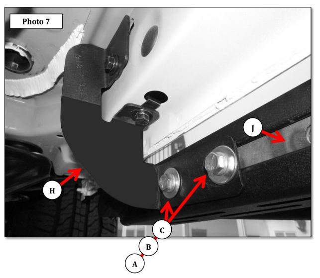
**Step-7** Align the running board with the vehicle and tighten all bracket and side step nuts and bolts,. Repeat the above steps to install the driver side brackets and running board. Remember to check and retighten the nuts and bolts every six months.
