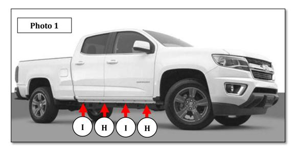
**Step-1** Begin the installation on the passenger side. Starting at the front of the vehicle, locate and remove the plastic plugs in the back side and bottom of rocker panel to expose the holes used for placement of the M8 Clip- Nuts, (Photo 2).
