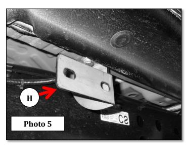
**Step-5** Insert four of the Nut-Plates through the rectangular opening in the back of the Dominator D6 running board. Measure and position each Nut-Plate so it aligns with one of the three mounting brackets previously attached to the vehicle, (Photo 6).
