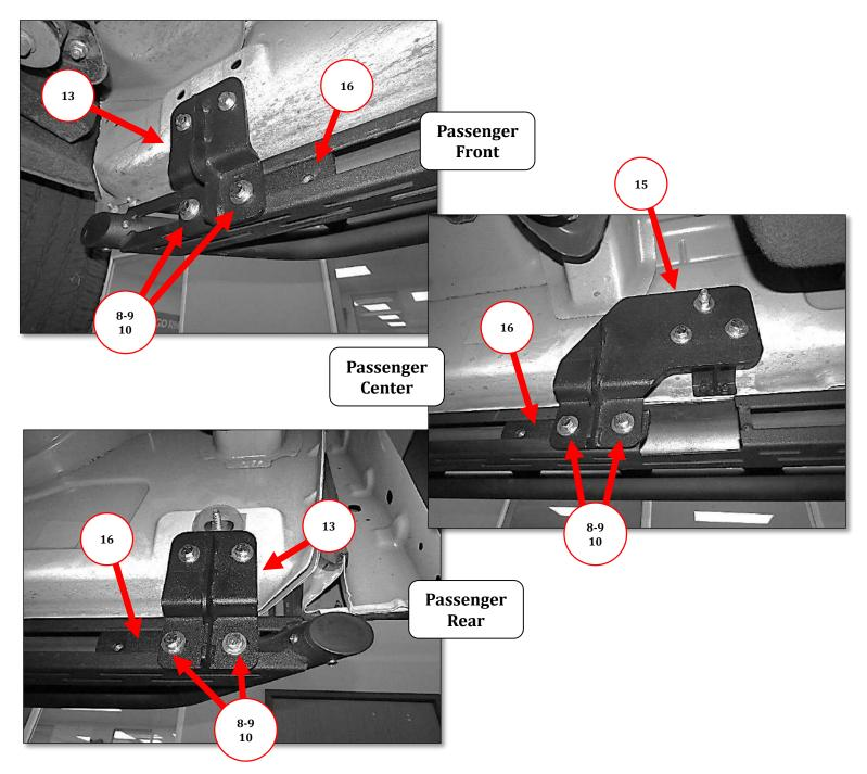
**Step-10** Tighten all bolts securing the Dominator D6 running board to the three brackets. Repeat the above steps to install the brackets and Dominator D6 running board on the driver side of the vehicle. Remember to check and retighten the nuts and bolts every six months.
