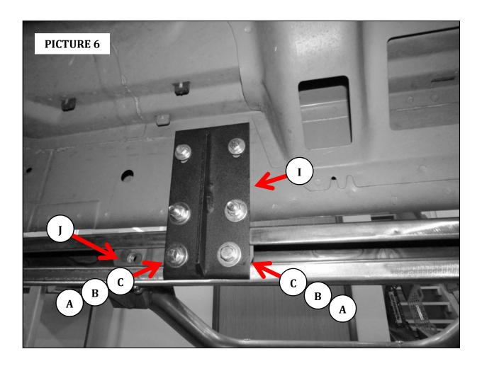
**Step-7** Align the running board with the vehicle and tighten all bracket and side step nuts and bolts,. Repeat the above steps to install the driver side brackets and running board. Remember to check and retighten the nuts and bolts every six months.
