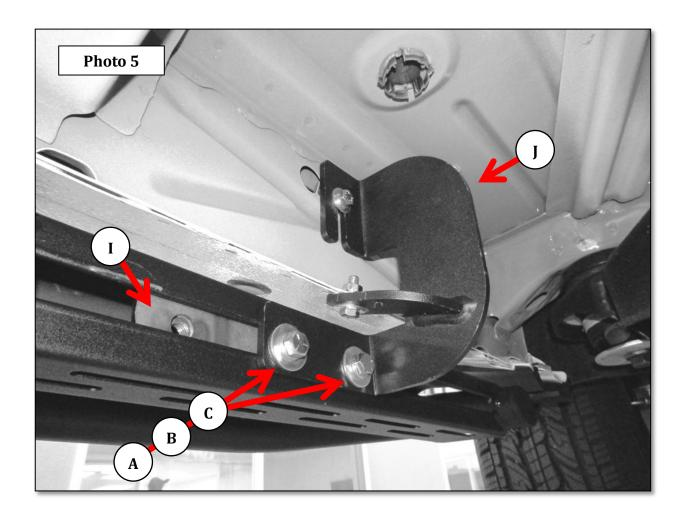
**Step-5** Align the running board with the vehicle and tighten all bracket and side step nuts and bolts,. Repeat the above steps to install the passenger side brackets and running board. Remember to check and retighten the nuts and bolts every six months.
