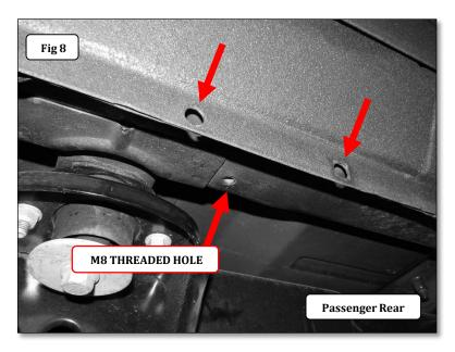
**Step-6** Attach the passenger side rear bracket to the pinch mold using (2) 5/16" x 1" button head bolts, (2) 5/16" flat washers, (2) 5/16" lock washers and (2) 5/16" hex nuts, and to the underside of the body using (1) M8 x 25mm hex bolt, (1) 5/16" lock washer and (1) 5/16" flat washer, (Fig 9 & 10). Leave the nuts and bolts loose for final adjustment.
