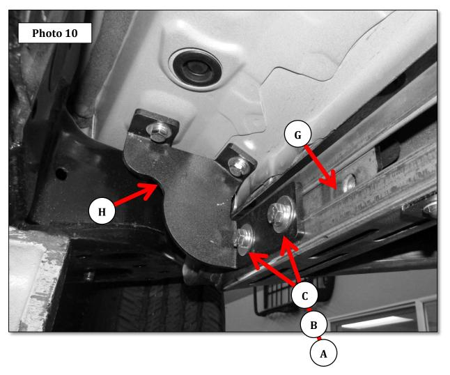
**Step-9** Align the Dominator D1 side step with the vehicle and tighten all bracket and side step nuts and bolts,. Repeat the above steps to install the brackets and Dominator D1 side step on the driver side of the vehicle.
