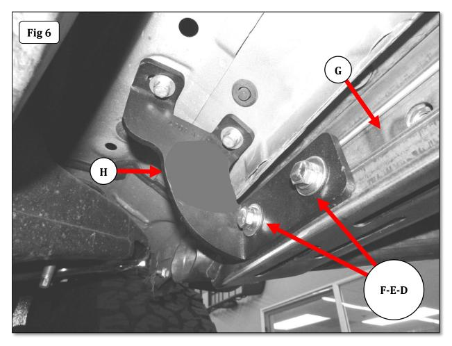
**Step-7** Align the Dominator D1 side step with the vehicle and tighten all bracket and side step nuts and bolts. Repeat the above steps to install the brackets and Dominator D1 side step on the driver side of the vehicle.
