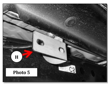
**Step-5** Insert four of the Nut-Plates through the rectangular opening in the back of the Dominator D1 side step. Measure and position each Nut-Plate so it aligns with one of the three mounting brackets previously attached to the vehicle, (Photo 6).
