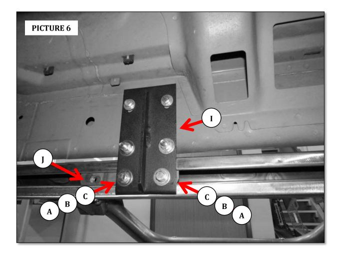
**Step-7** Align the Dominator D1 side step with the vehicle and tighten all bracket and side step nuts and bolts,. Repeat the above steps to install the brackets and Dominator D1 side step on the driver side of the vehicle.
