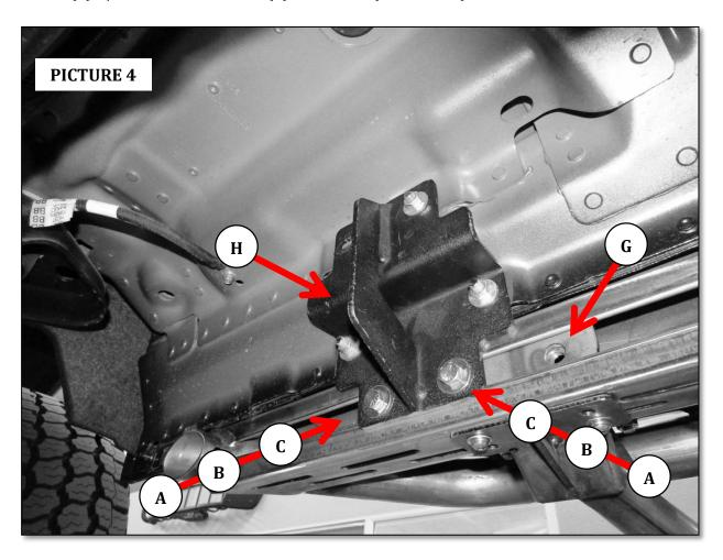
**Step-5** Align the Dominator D1 side step with the vehicle and tighten all bracket and side step nuts and bolts,. Repeat the above steps to install the driver side brackets and Dominator D1 side step.
