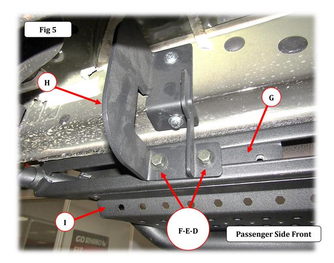
**Step-6** Tighten the bolts securing the mounting brackets to the body panel and the bolts securing the Dominator D1 side step to the mounting brackets.
