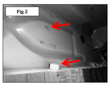
**Step-2** Attach one of the driver side brackets to the pinch mold using (1) M8 hex bolt, (1) 5/16" lock washer and (1) 5/16" lock washer, and to the rocker panel using (1) M8 hex bolt, (1) 5/16" lock washer and (1) 5/16" flat washer. Leave the bolts loose for final adjustment, (Fig 3).
