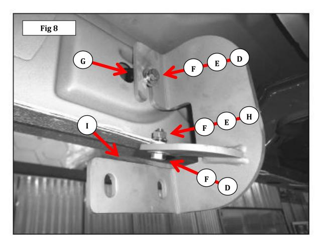
**Step-5** Install the driver side rear bracket by measuring from the front fender bolt reward approximately 75 1/8" and repeat the above steps.
