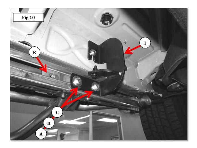
**Step-8** Align the D1 side step with the vehicle and tighten all bracket and side step nuts and bolts,. Repeat the above steps to install the brackets and D1 side step on the passenger side. Remember to check and retighten the nuts and bolts every six months.
