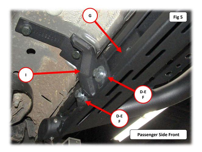
**Step-6** Align the Dominator D1 side step with the vehicle and tighten all bracket and side step nuts and bolts,. Repeat the above steps to install the driver side brackets and Dominator D1 side step.
