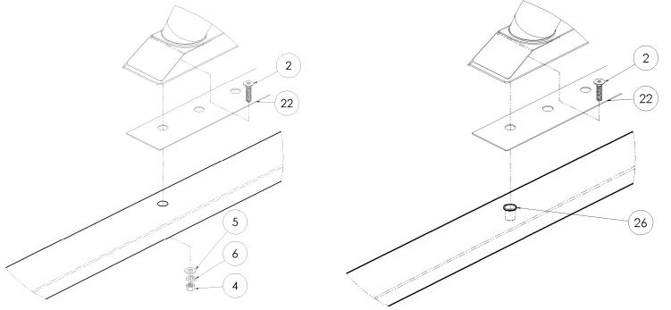
Tighten all front and rear tube bolts to 26 ft/lbs Max. DO NOT OVERTIGHTEN BOLTS
