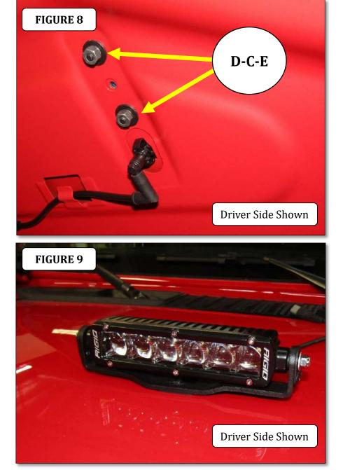
**Step-14** Repeat the above steps to install the LED light and bracket assembly on the passenger side of the vehicle. Re-install the insulator panel to the underside of the hood using the supplied plastic tree clips.
