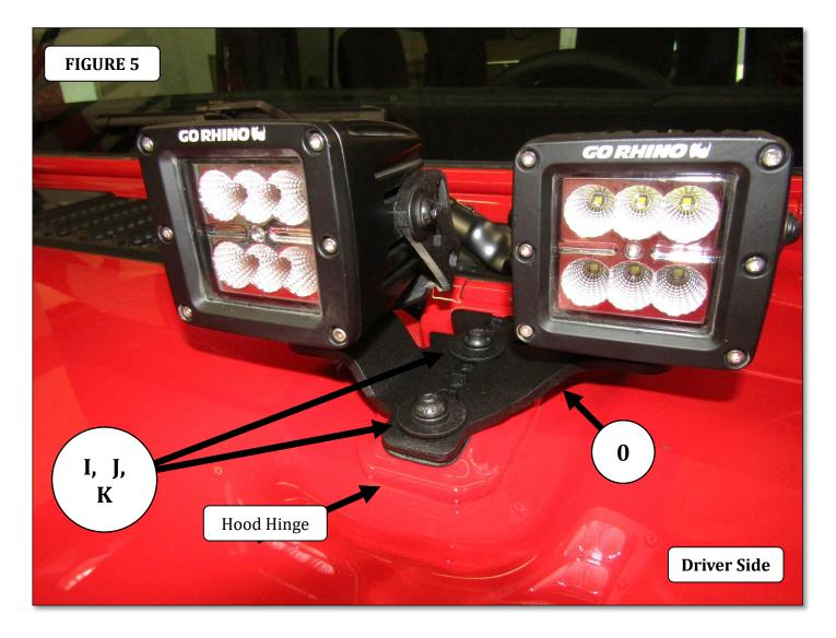
**Step-6** Adjust the LED lights and light brackets so the lens of the LED lights are in the desired position, then tighten all screws and bolts.
