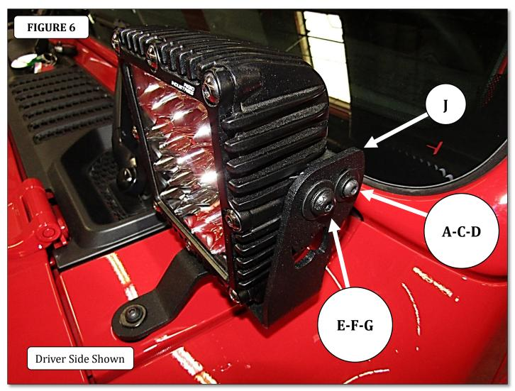
**Step-6** Repeat the above steps to install the cowl light mount bracket and Q-4 Series light on the passenger side of the vehicle.
