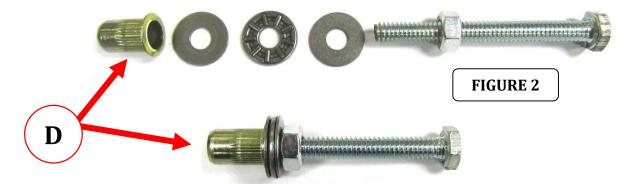
**Step-4** Place the rivet-nut with the attached tool components into the enlarged hole in one of the tabs. Use a 7/16" wrench to hold the nut, and tighten the bolt using a 7/16" wrench or socket and ratchet. Continue tightening the bolt until the rivet-nut is fully compressed and no longer spins then remove the tool components, (FIGURE 3). Repeat for the enlarged hole in the remaining tab.
