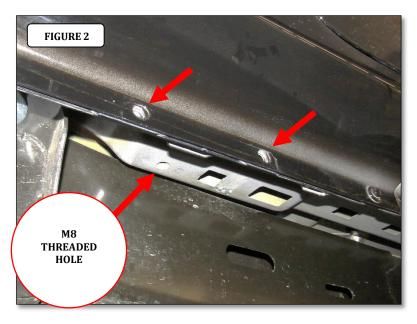
**Step-2** Attach one of the driver side Front/Front Center brackets to the pinch mold using (2) 1/4" x 1" hex head bolts, (4) 1/4" flat washers, (2) 1/4" lock washers and (2) 1/4" hex nuts, and to the underside of the body using (1) M8 x 25mm hex bolt, (1) 5/16" lock washer and (1) 5/16" flat washer, (FIGURE 3 & 4). Leave the nuts and bolts loose for final adjustment.
