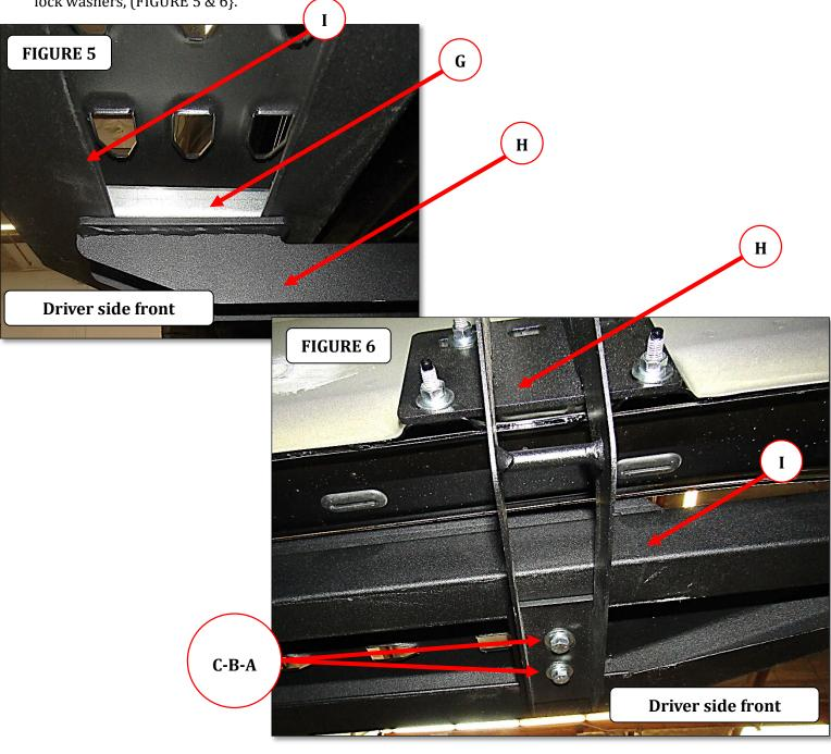
**Step-5** Align the running board with the vehicle and tighten all supplied nuts and bolts securing the running board and bracket assembly. Repeat to install the passenger running board.
