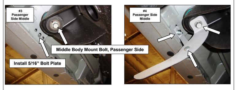
**Step-5** Remove the passenger side rear body mount bolt. Keep all existing washer and bushing in place, and attach the passenger side rear bracket to the vehicle using the factory body mount bolt and supplied ½" flat washer, (Photo 5 & 6). Leave the body mount bolt loose for final adjustment.
