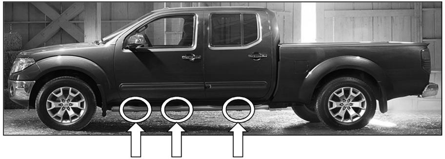
In this part, under the vehicle install the driver side front, middle and rear bracket.
