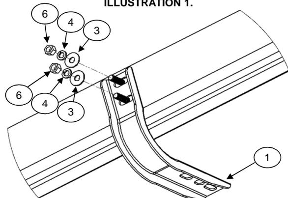
6.- If you acquired a 5" or 6" COMPOSITE Side bar, insert 5/16" square head bolt on rail, place on brackets and attach with: 5/16" Flat and lock washer, 5/16" hex nut. **SEE ILLUSTRATION 2.** Repeat for the opposite side. Leave loose.
