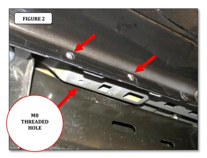
**Step-2** Attach one of the driver side Front/Center brackets to the pinch mold using (2) 1/4" x 1" hex head bolts, (4) 1/4" flat washers, (2) 1/4" lock washers and (2) 1/4" hex nuts, and to the underside of the body using (1) M8 x 25mm hex bolt, (1) 5/16" lock washer and (1) 5/16" flat washer, (FIGURE 3 & 4). Leave the nuts and bolts loose for final adjustment.
